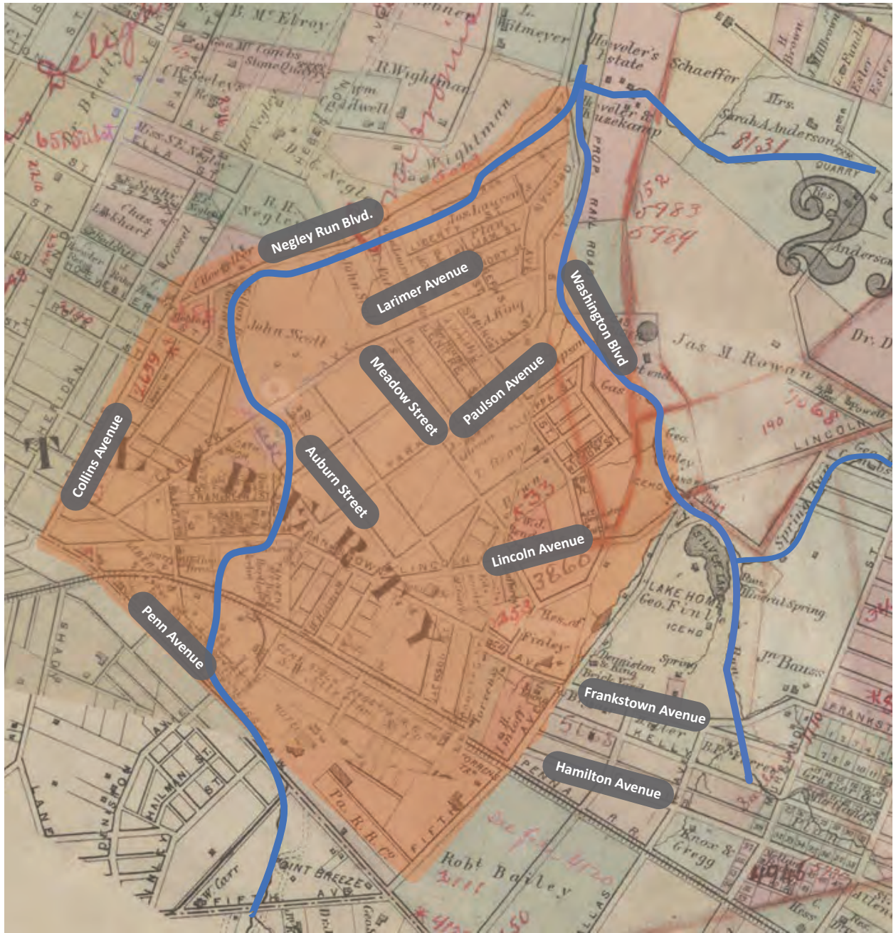
Fig. 35 Historic Drainage This map shows the historic waterways in the Larimer neighborhood. These are no longer present as surface water ways, but suggest where historic drainages could be recreated as part of a green infrastructure system.
